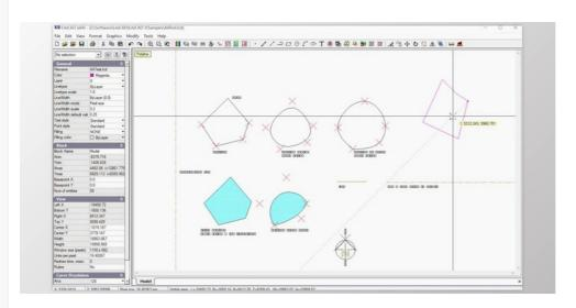
LiteCAD SDK allows software developers to create specialized drawing applications. It is CAD/CAM/GIS compatible. The package's main component, LiteCAD DLL, provides 2D vector graphics and an API with popular languages like C++, C# VB6 VB.NET, Delphi. The OCX module provides an ActiveX interface to the DLL. The SDK includes a powerful CAD editor that is based entirely upon the LiteCAD DLL.
