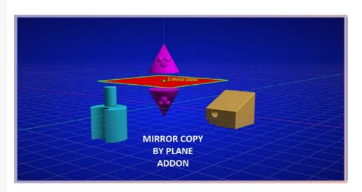
With this extension, you can easily create a mirror image of an object with the use of the plane.
