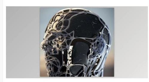
Smooth Subdivision enlarges the geometry of your design by adding polygons. Linear Subdivision is performed prior to Smooth subdivision and is employed to highlight edges.
